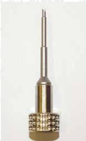
Fig. 2. Screw removal instrument (Lucky, SC-1713, ADL Bio, Seoul, Korea). The sharp-edged tips of the screw removal instrument can engage the irregular top surfaces of fractured screw fragments.
