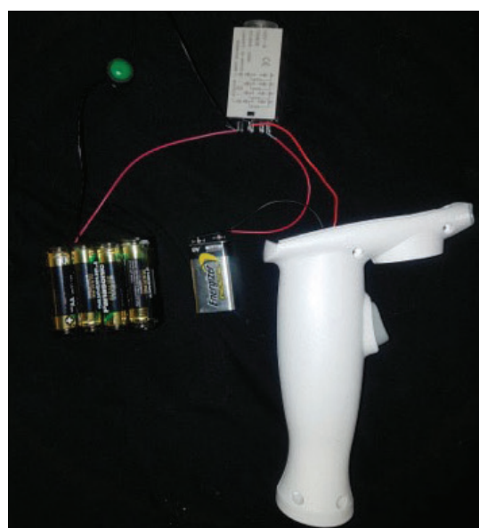
Figure 3. Time limit relay connected to the powder spraying machine
